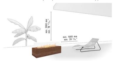
Fig. 1: Minimum distance to flammable materials
