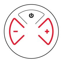
Pressing the "+" button twice automatically increases the flames to the HIGH position
