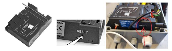
Fig. 7 - Receiver "RESET" button
